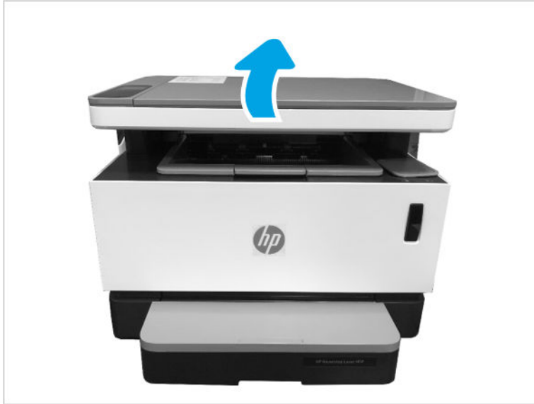
Figure 1-106 Open the image scanner assembly
