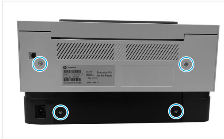
Figure 1-44 Remove four screw
