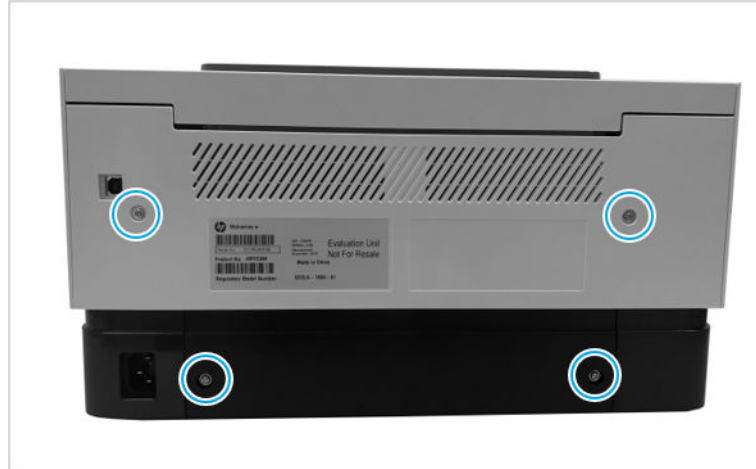
Figure 1-218 Remove four screw
