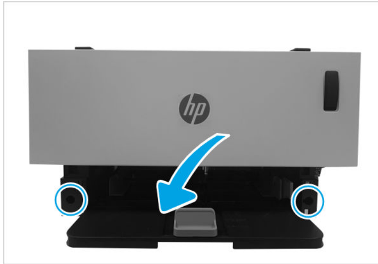
Figure 1-194 Remove front cover
