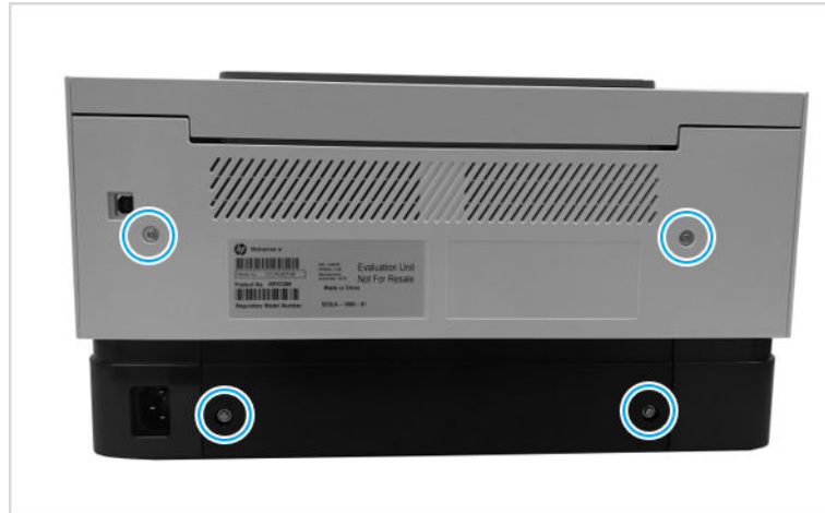
Figure 1-131 Remove four screw
