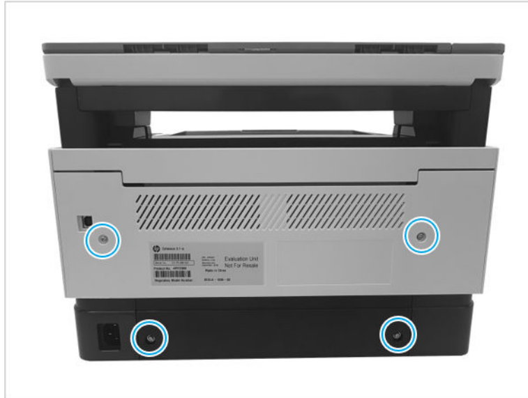
Figure 1-151 Remove four screw
