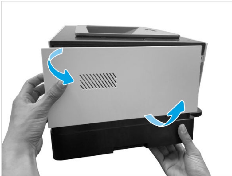
Figure 1-285 Remove left cover
