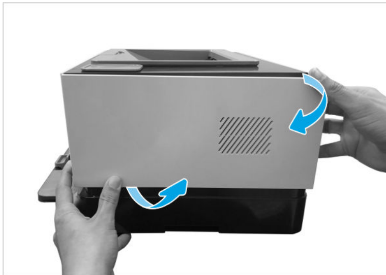
Figure 1-82 Remove right cover
