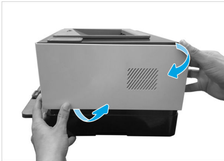
Figure 1-166 Remove right cover
