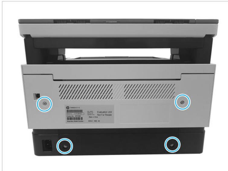
Figure 1-288 Remove four screw
