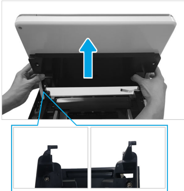
Figure 1-253 Remove the image scanner assembly
