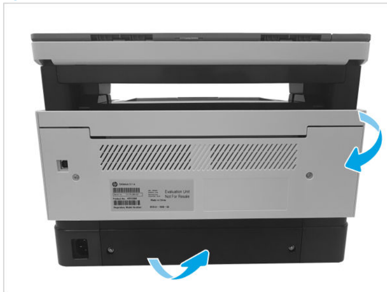
Figure 1-182 Remove rear cover
