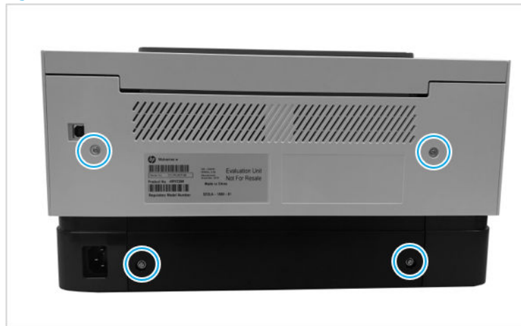
Figure 1-38 Remove four screw
