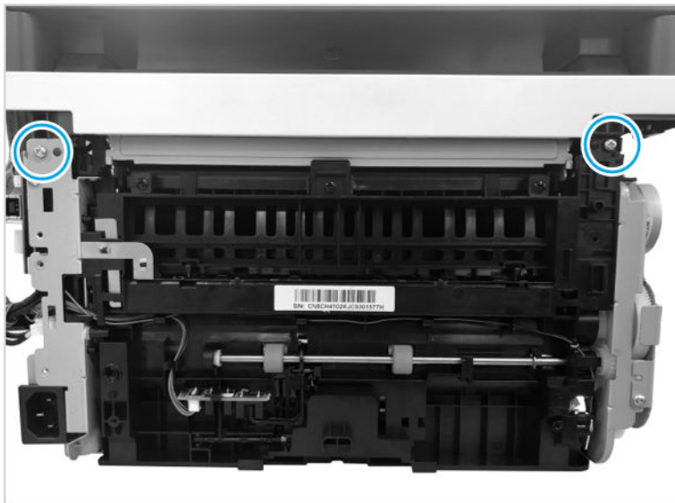
Figure 1-197 Remove the two screws
