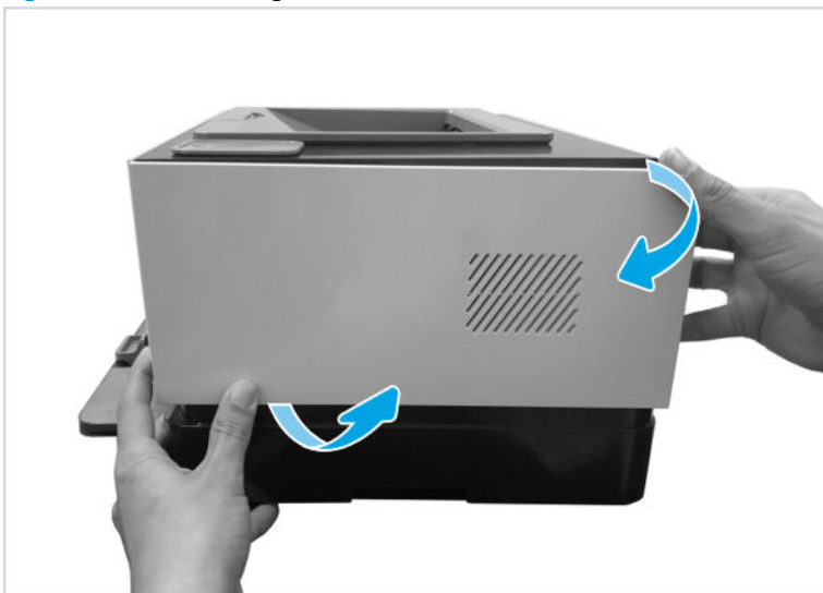
Figure 1-64 Remove right cover
