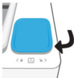
Figure 1-8 Cover the reload port
