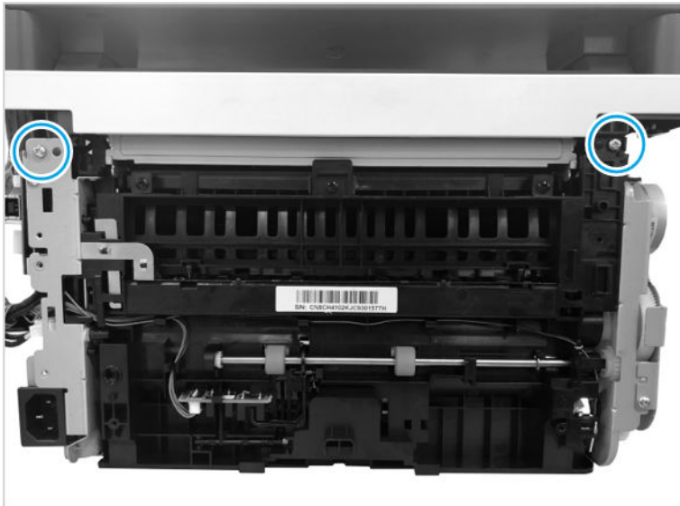
Figure 1-260 Remove the two screws
