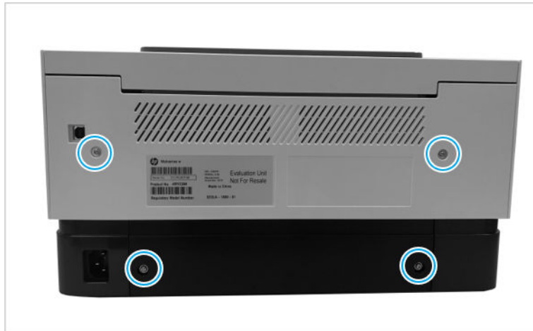
Figure 1-282 Remove four screw
