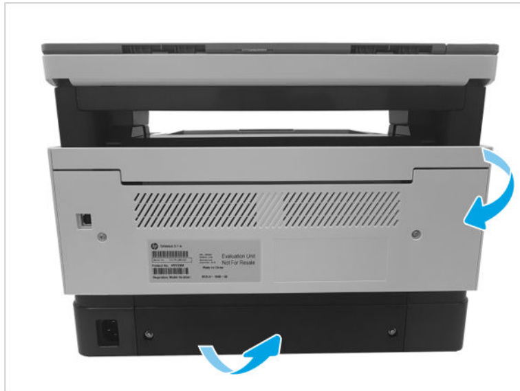
Figure 1-71 Remove rear cover
