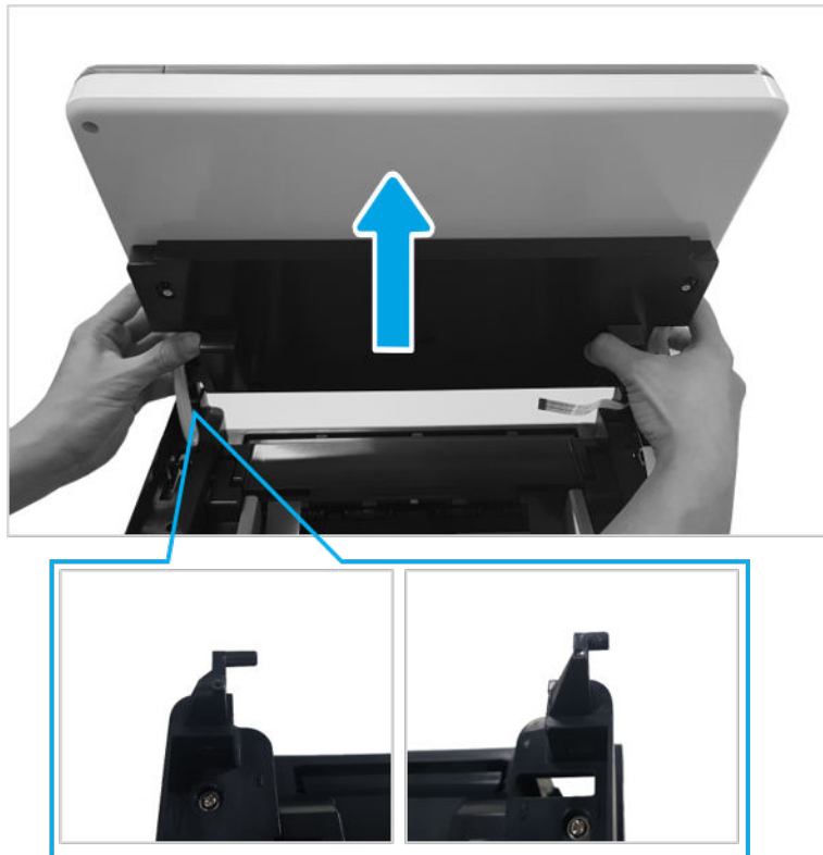
Figure 1-99 Remove the image scanner assembly
