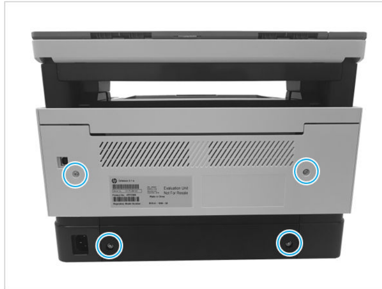
Figure 1-136 Remove four screw
