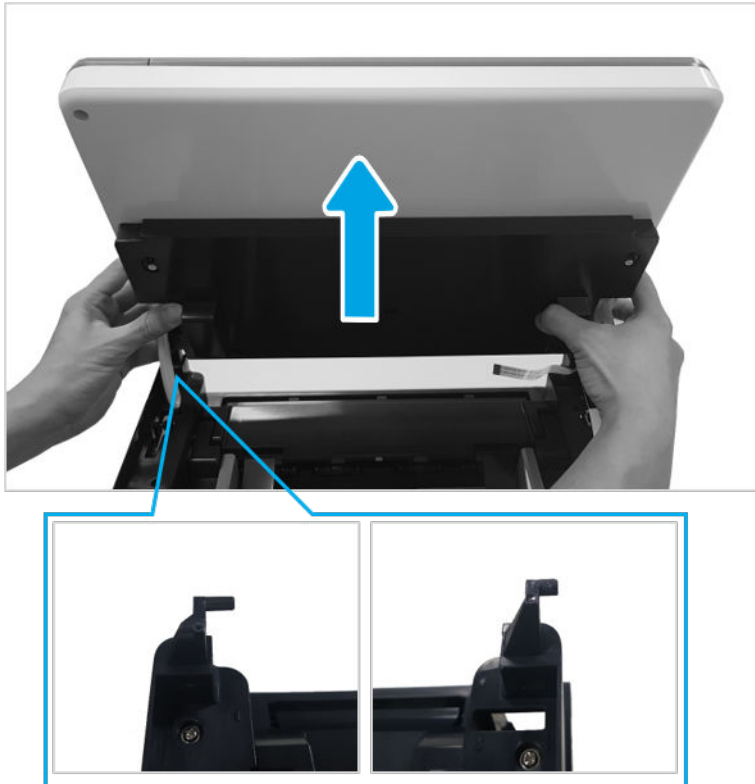
Figure 1-110 Remove the image scanner assembly
