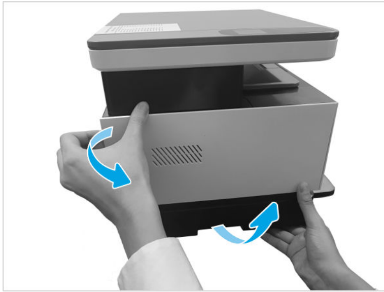
Figure 1-246 Remove left cover
