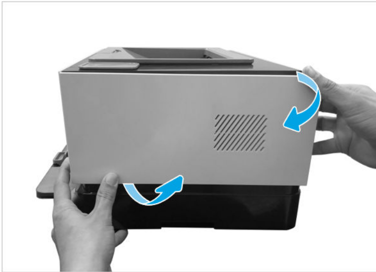
Figure 1-122 Remove right cover
