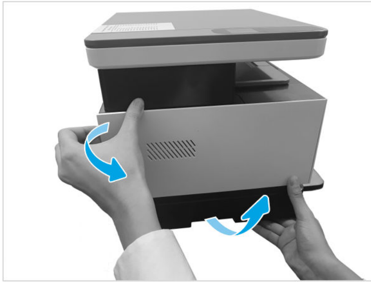
Figure 1-183 Remove left cover
