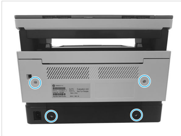
Figure 1-211 Remove four screw
