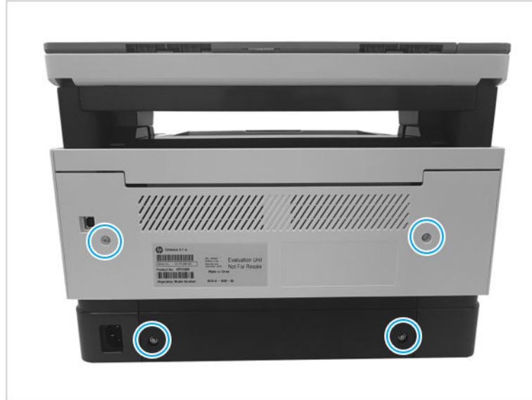
Figure 1-305 Remove four screw
