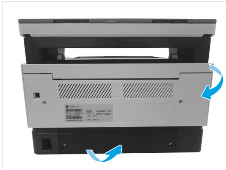
Figure 1-245 Remove rear cover
