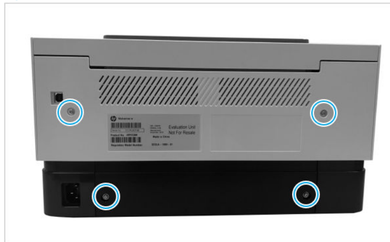
Figure 1-141 Remove four screw
