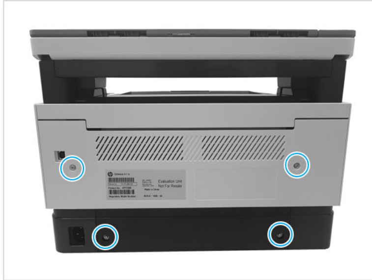
Figure 1-100 Remove four screw
