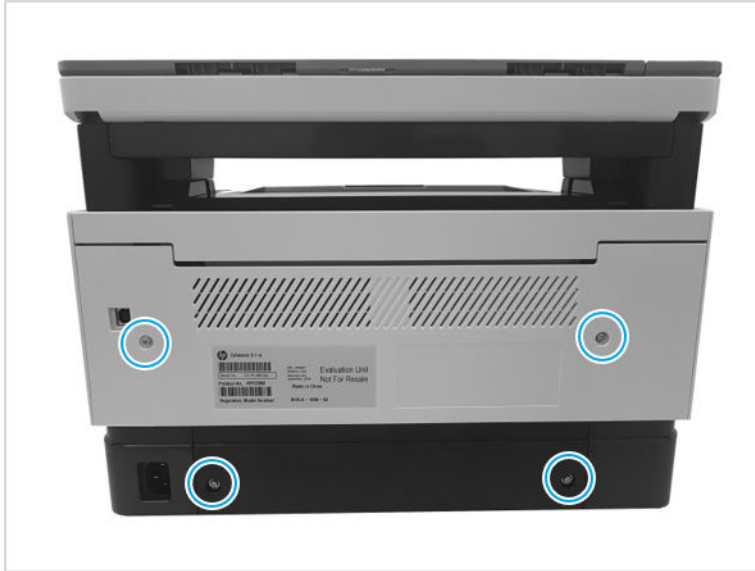
Figure 1-69 Remove four screw
