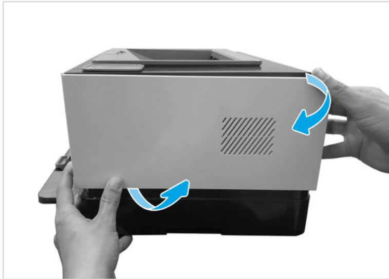
Figure 1-134 Remove right cover
