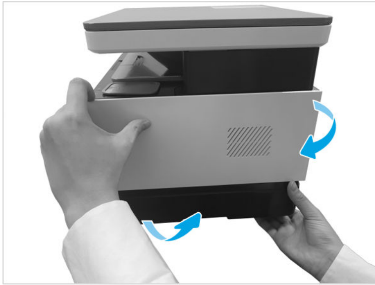
Figure 1-73 Remove right cover
