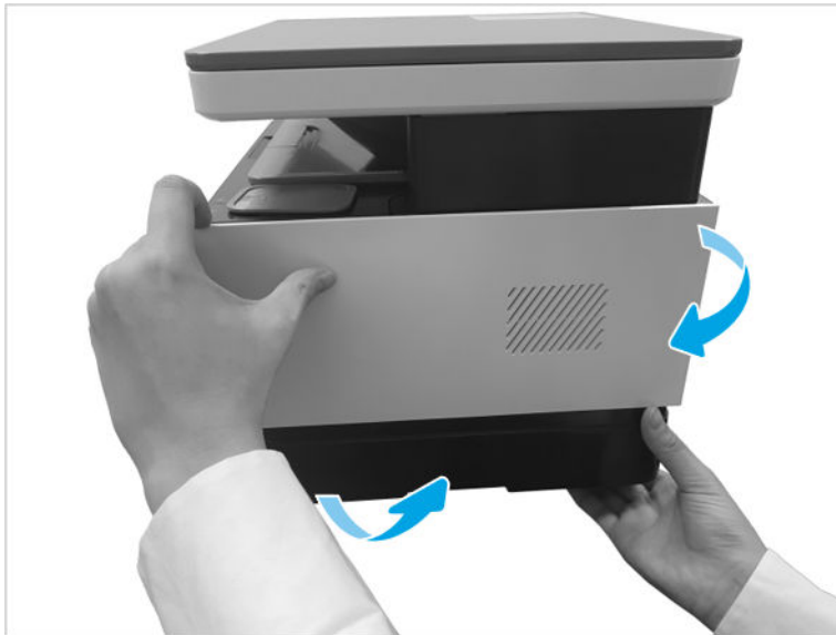
Figure 1-104 Remove right cover
