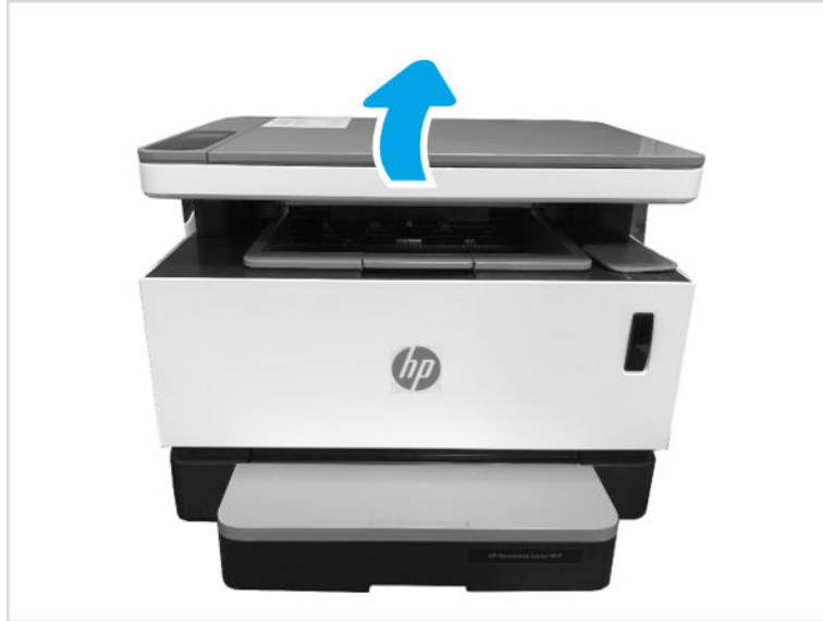
Figure 1-249 Open the image scanner assembly
