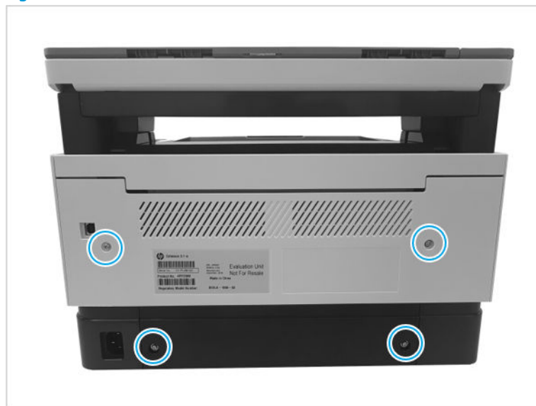
Figure 1-125 Remove four screw
