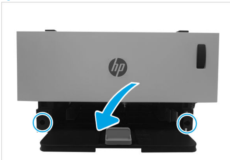
Figure 1-68 Remove front cover
