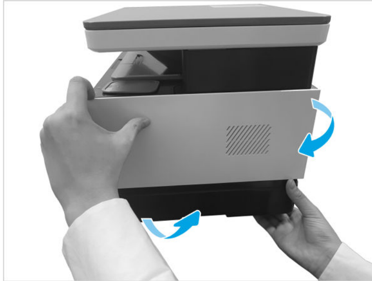
Figure 1-93 Remove right cover
