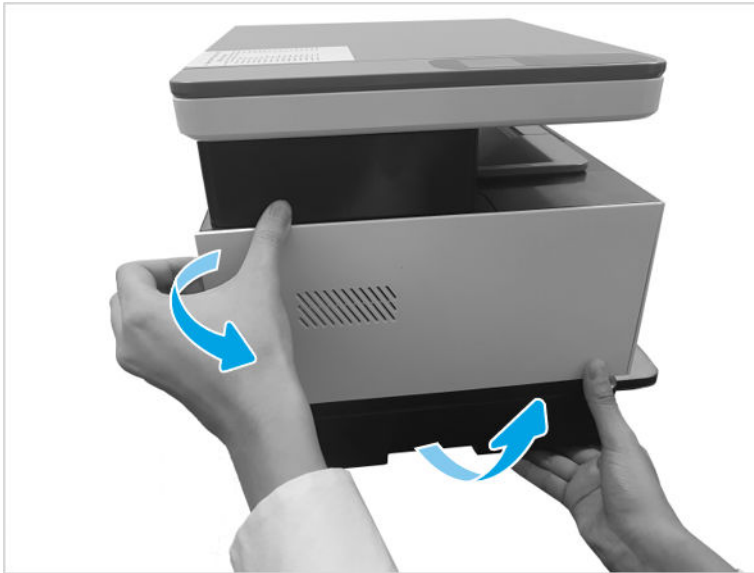
Figure 1-291 Remove left cover
