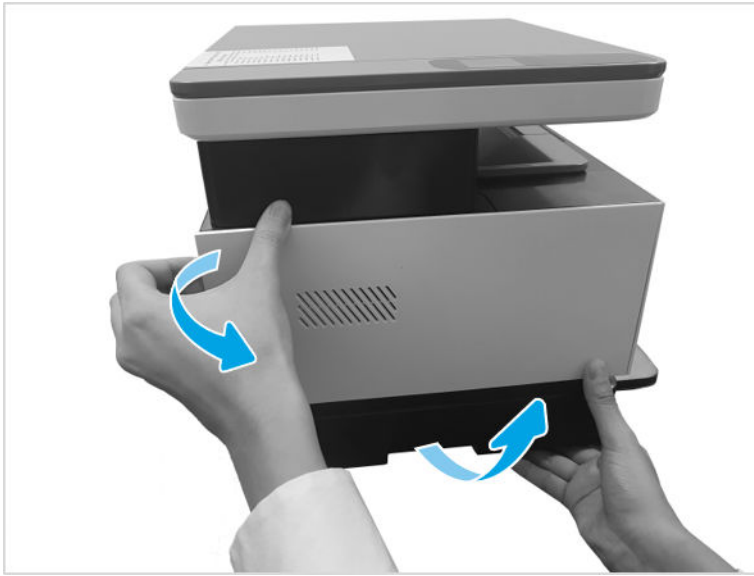
Figure 1-103 Remove left cover
