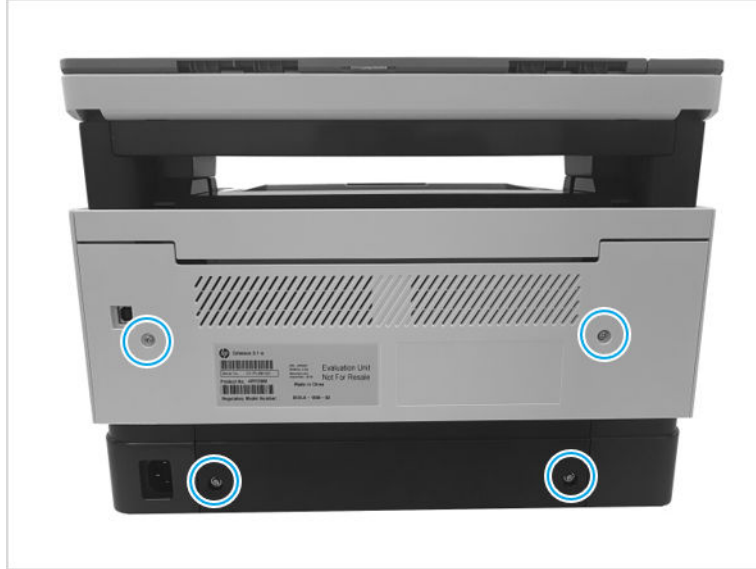
Figure 1-90 Remove four screw
