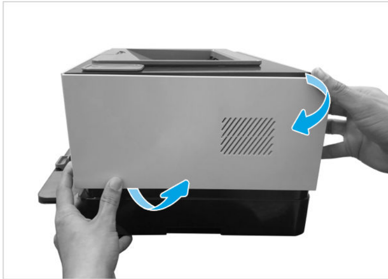
Figure 1-47 Remove right cover
