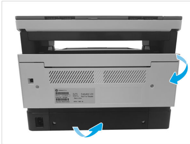
Figure 1-153 Remove rear cover
