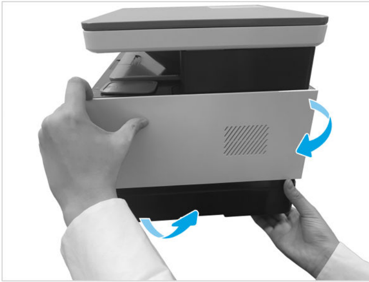
Figure 1-51 Remove right cover
