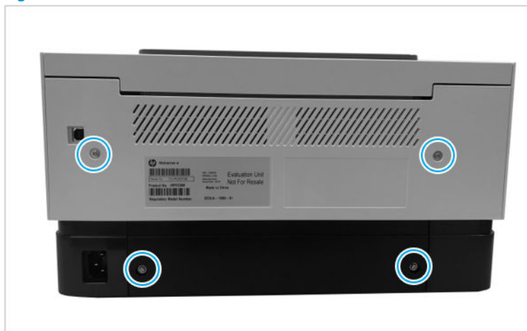
Figure 1-119 Remove four screw
