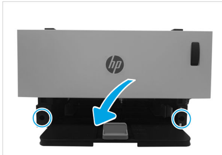
Figure 1-257 Remove front cover
