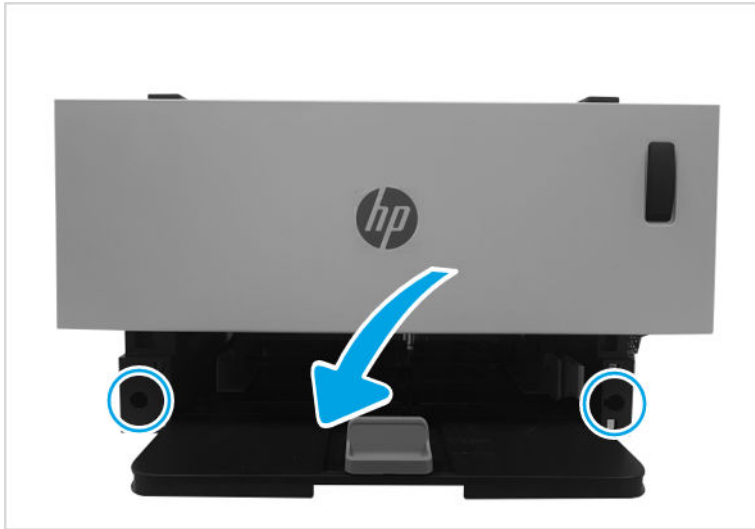
Figure 1-114 Remove front cover
