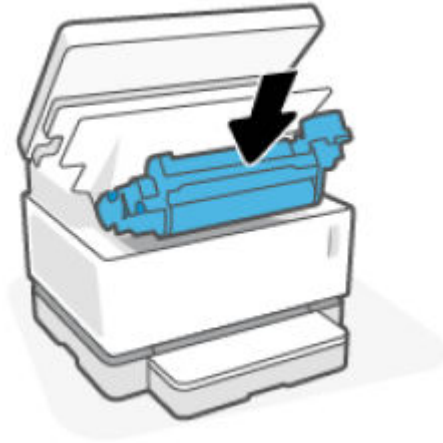
Figure 1-36 Insert the new imaging drum
