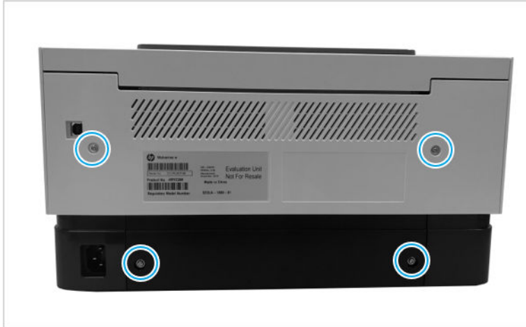
Figure 1-205 Remove four screw
