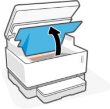
Figure 1-33 Lift the top cover
