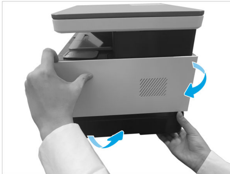
Figure 1-247 Remove right cover
