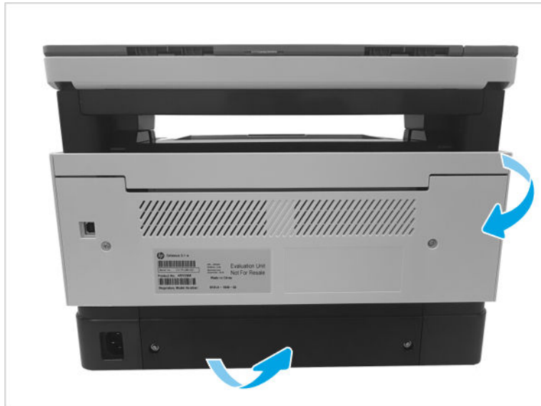
Figure 1-58 Remove rear cover
