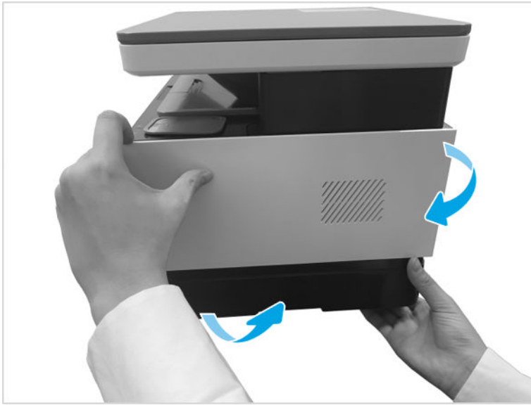
Figure 1-128 Remove right cover
