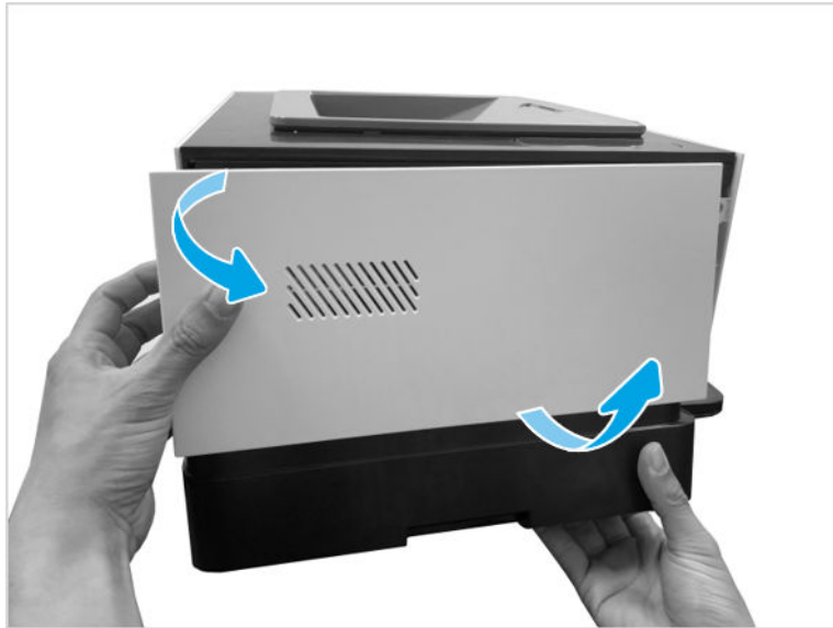
Figure 1-81 Remove left cover
