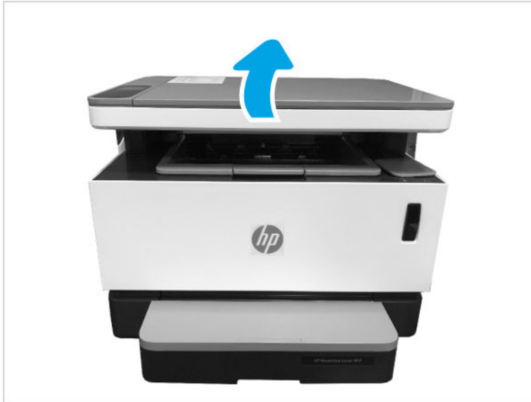
Figure 1-95 Open the image scanner assembly
