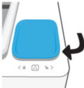
Figure 1-20 Cover the reload port
