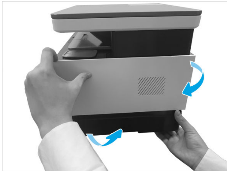
Figure 1-184 Remove right cover
