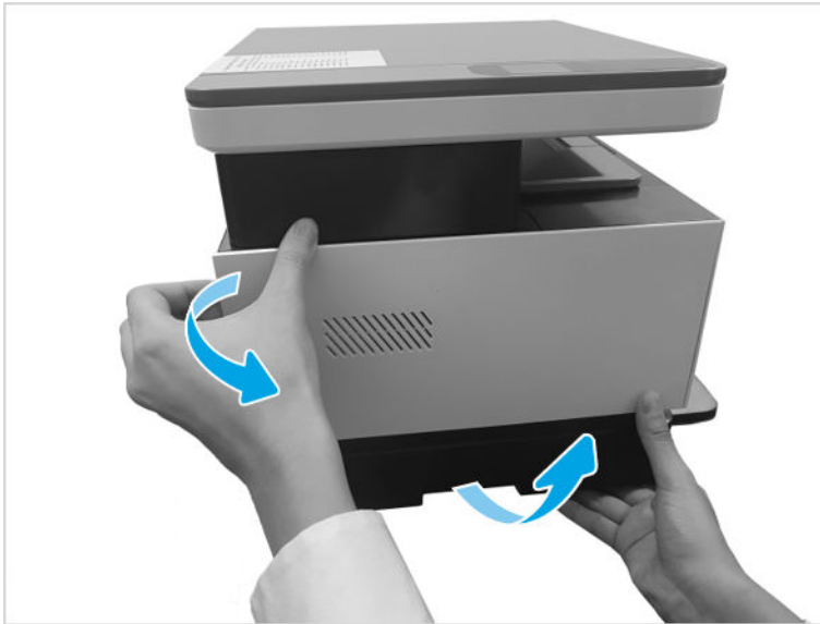
Figure 1-214 Remove left cover
