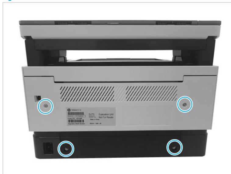
Figure 1-180 Remove four screw
