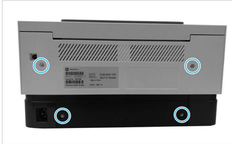
Figure 1-162 Remove four screw
