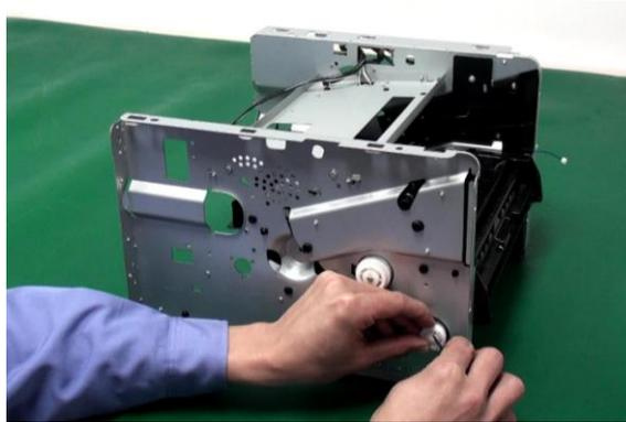
2. Remove the spring and the dowel.
