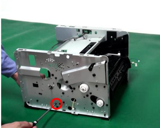
2. Unscrew the screw fixed to the motor and remove the motor.
