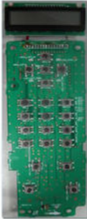
Figure 1-26 Control panel PCA image (HP Laser MFP 432fdn)
