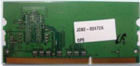
Figure 1-27 SO-DIMM PCA
