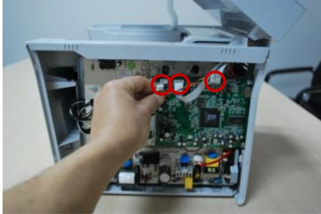
2. Separate the scan bracket and the scanning platform.
