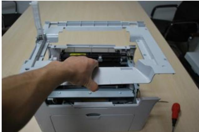
5. After removing the upper cover, take out the rear cover screws.
