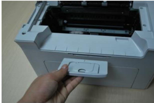
3. After removing the output bin, take out the upper cover screws.
