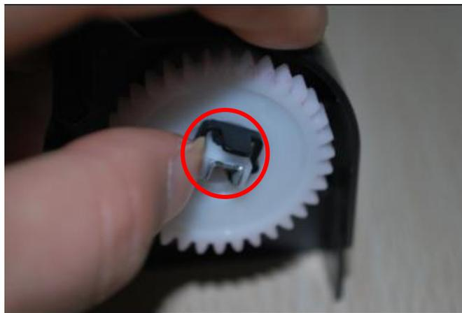
8. Remove the clutch gear.
