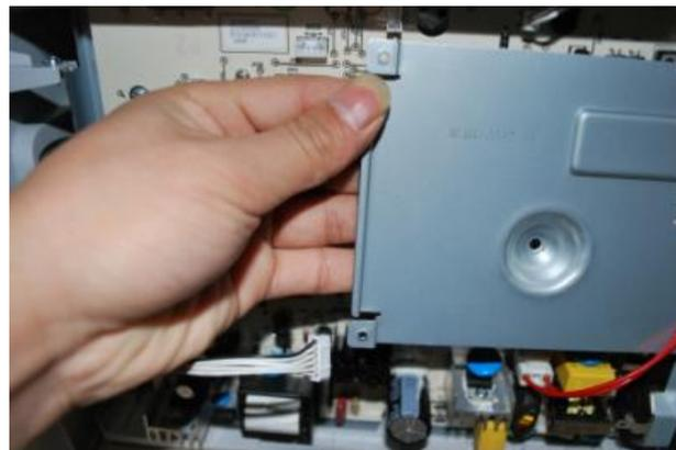
4. After removing the data board fixing plate, unplug the cable, as shown in the figure.
