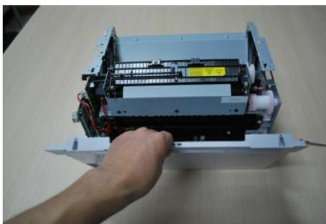
7. After removing the upper cover, take out the front cover screws.
