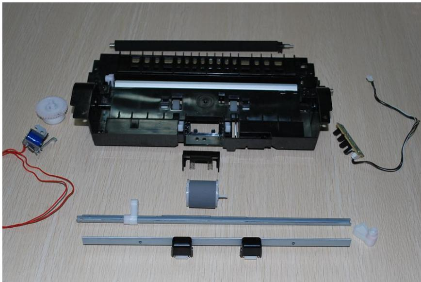
2. After removing the transportation components, open the claw on the right side of the transfer roller.
