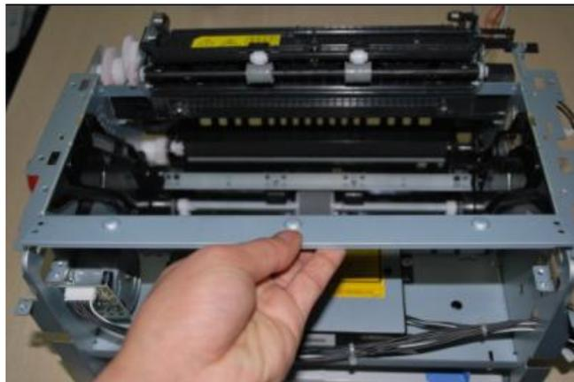
3. Unplug the main motor and the laser cable.
