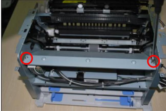
2. Remove the shield on the laser.
