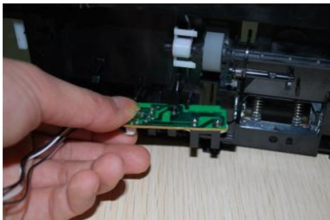
11. Remove the transport bracket screws, then take out the transport bracket.
