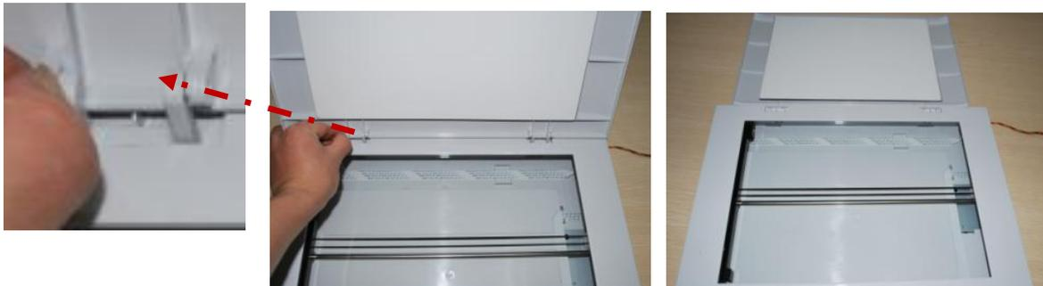
3. Remove the operation panel fixing screws.
