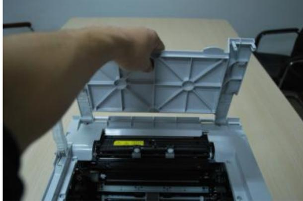
2. Remove the components of the delivery tray.
