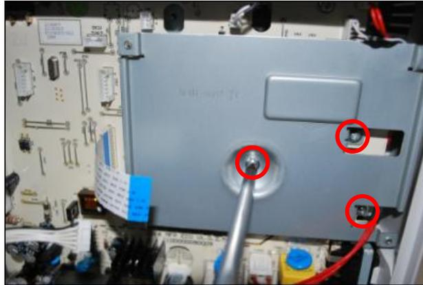
3. Remove the data board fixing plate.
