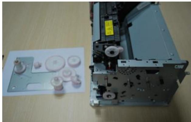
3. Unscrew the fuser fixing screws.
