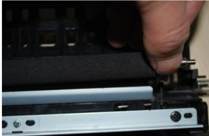
4. Take out the induction substrate and the electromagnet cable from the card slot.
