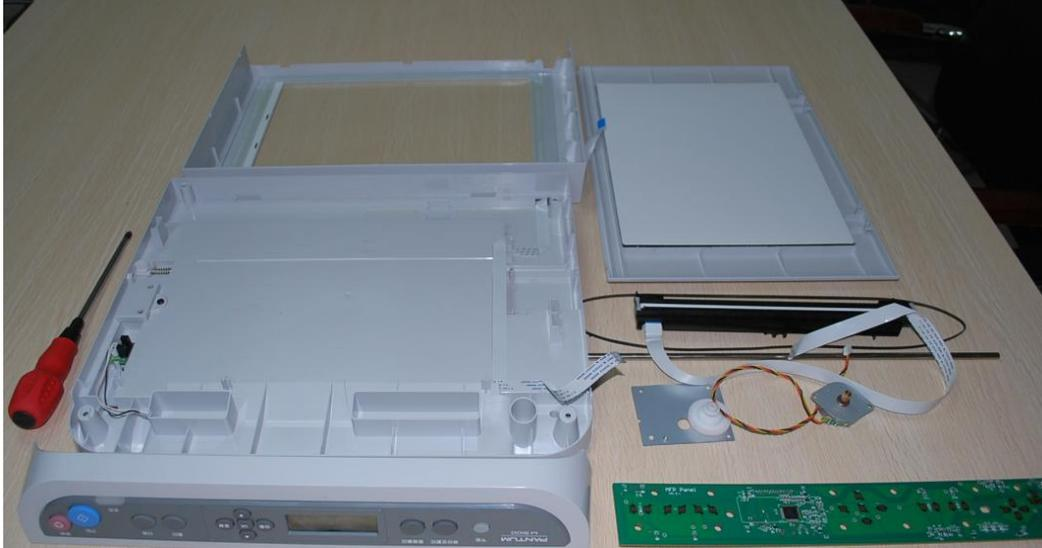
2. After removing the scanning platform, release the scanner cover connectors and take off the scanner cover.
