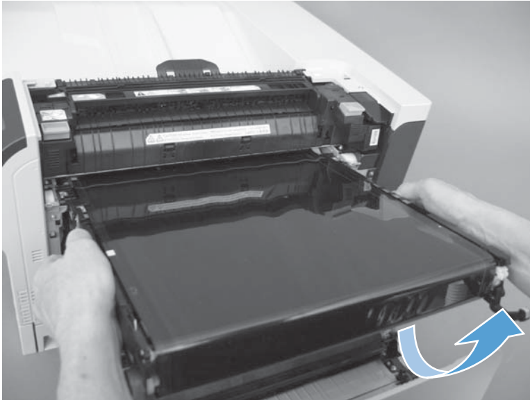
Figure 2-18 Remove the intermediate transfer belt (3 of 3)
