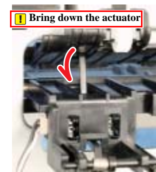
Figure 4-79. Removing the Upper Paper Guides
