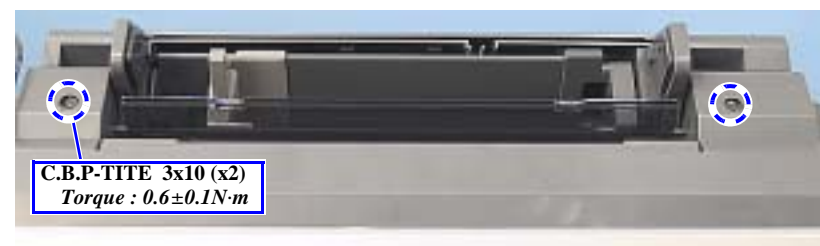
Figure 4-9. Removing the Scanner Unit
