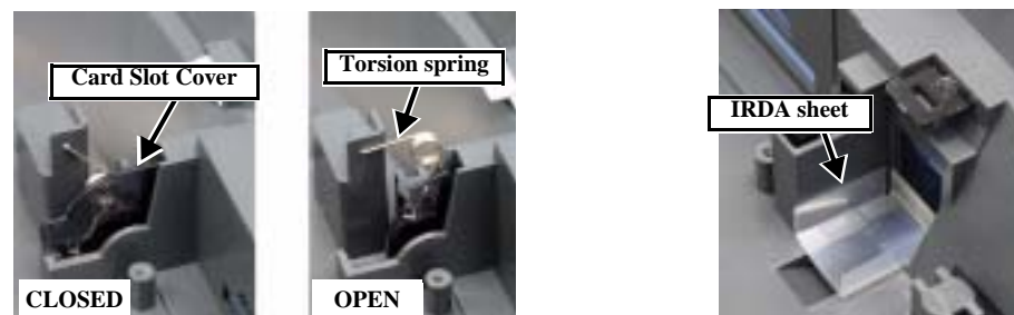
Figure 4-14. Checking the Middle Housing
