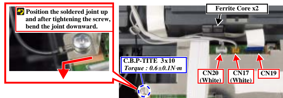
Figure 4-8. Disconnecting the cables (Scanner Unit)
