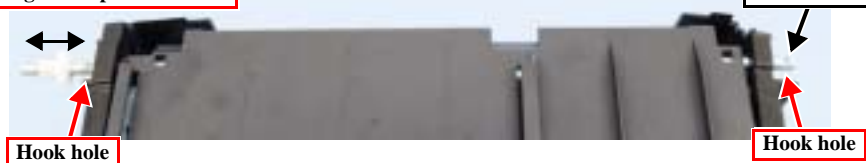
Figure 4-44. Installing the CD-R Shaft
