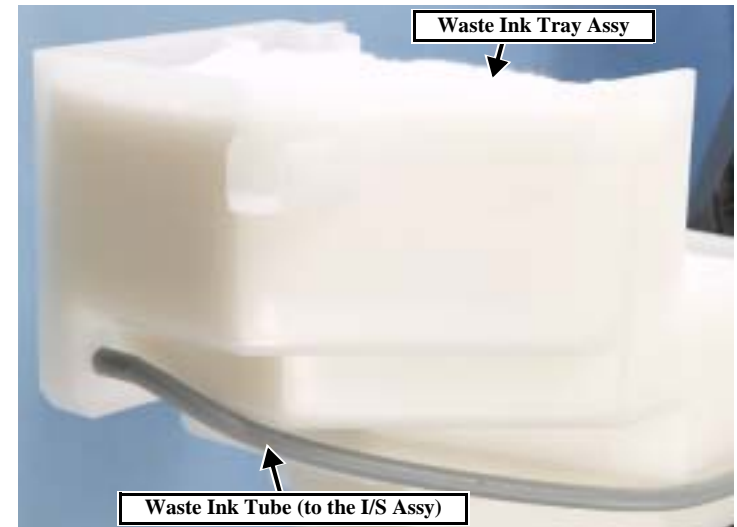
Figure 4-28. Removing the Waste Ink Tray Assy
