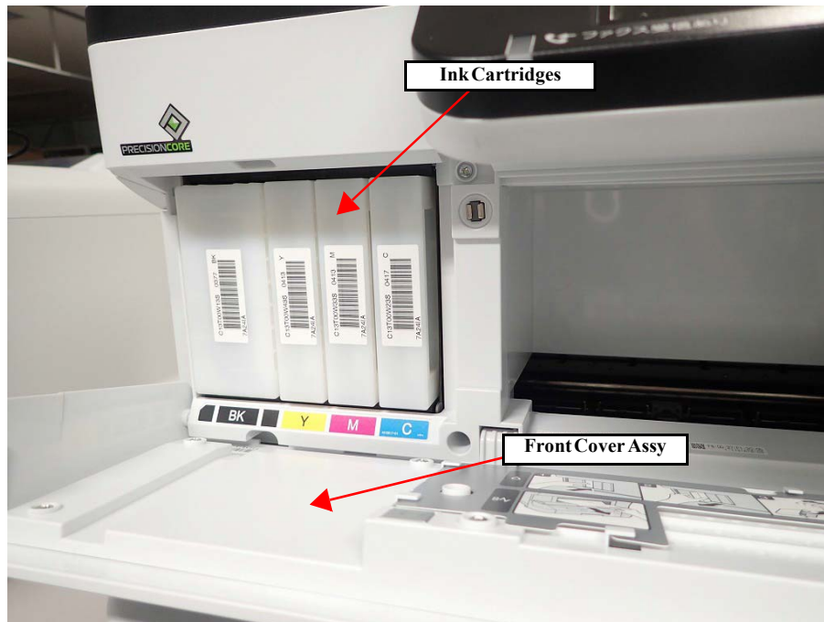
Figure 7-63. Removing the Ink Cartridge
