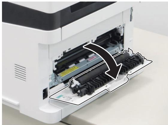
2. Remove the Secondary Transfer Roller.
