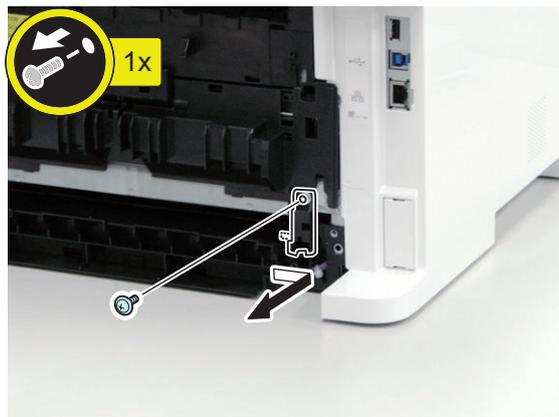
3. Remove the Secondary Transfer Feed Unit.
