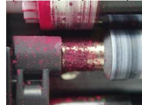
(Grease) \*applied inside the main charger roller bushing
